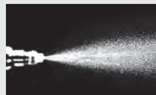
Injector spray pattern after P.i. treatment.
