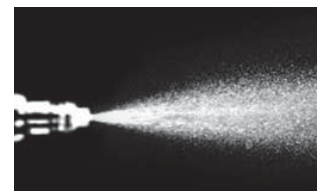
Injector spray pattern after P.i. treatment.
